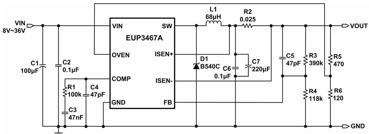
Figure 1. Application Circuit
