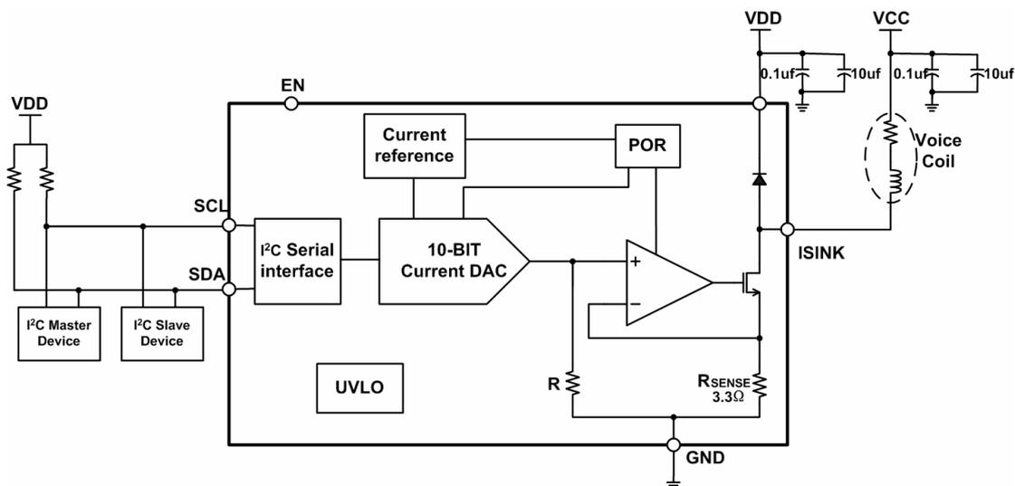
Figure 1. Application Circuit
