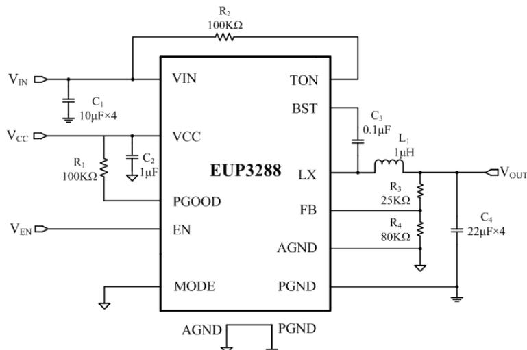
Figure 1. Application Circuit
