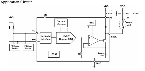
Figure 1. Application Circuit
