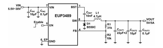
Figure 1. 5V Application Circuit
