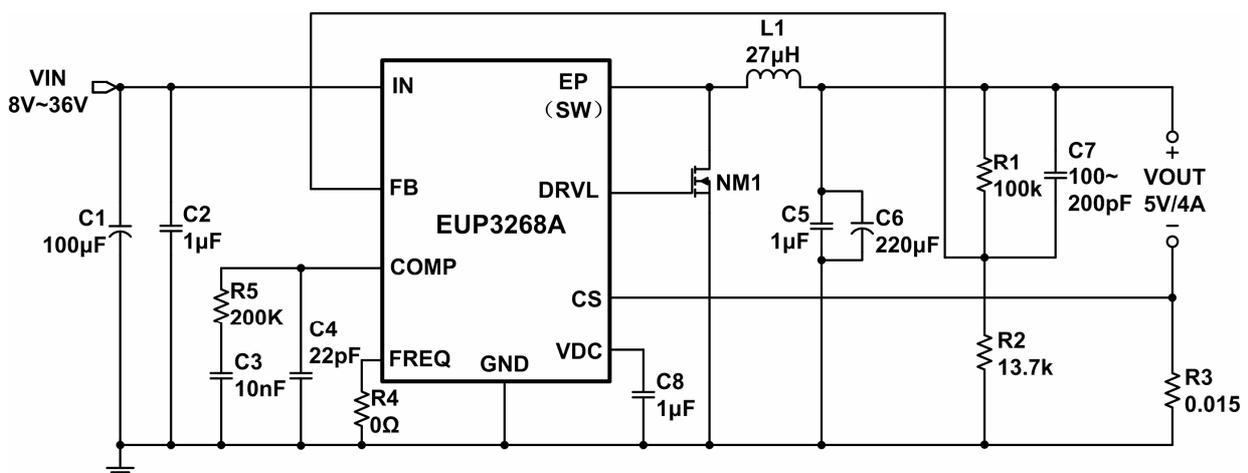
Figure 1. Application Circuit
