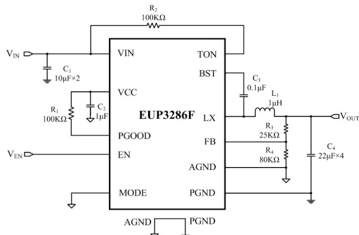
Figure 1. Application Circuit
