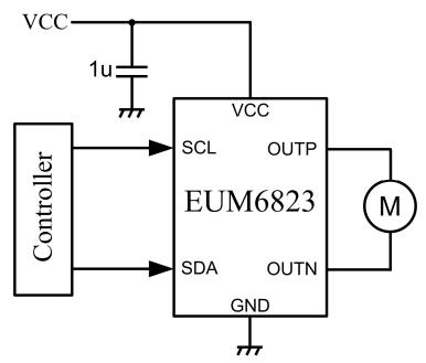
**Figure 1 Typical Application Circuits**
