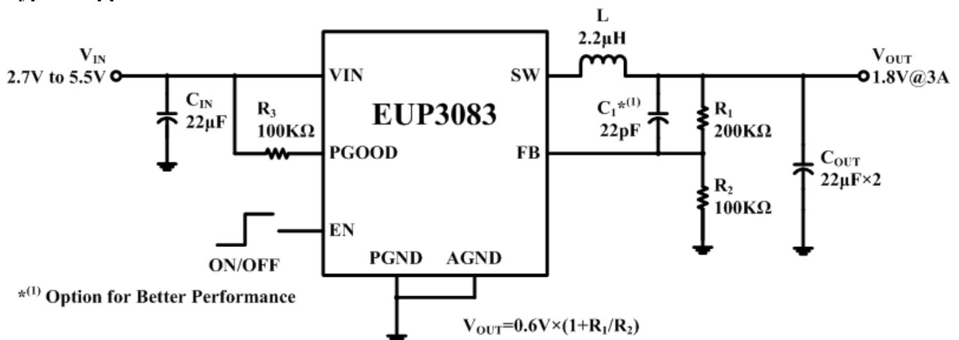
Figure 1. Application Circuit
