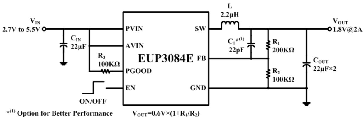
Figure 1. Application Circuit
